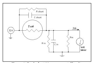
Figure 1. Equivalent Measurement Circuit.
